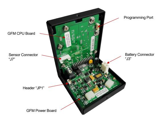
Inside View of GFM Enclosure (Power Board - Revision: A)
